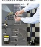
The Gen4 Model 8910 Instant Static Elimination Station removes contaminants on plastic fittings prior to packaging.
